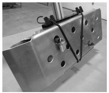
3. **Place Ramps on Rack** – After the carrying rack is securely mounted, the ramps are placed on the rack as shown at left. Stretch the two ends of the bungee cord across the ramps to the hook points. A padlock with up to a 5/16" shank can be inserted through one of the support fingers for security. The holes at the bottom of the rack provide a place to store the padlock when not in use.
