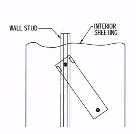
Enclosed Trailer Wall Mounting- Locate a wall stud and drill a 1/8" diameter hole. Use one No. 14 sheet metal screw to mount the top end of the scabbard and the metal bracket to the wall stud. Use the other No. 14 screw to mount the opposite end to the wall.
