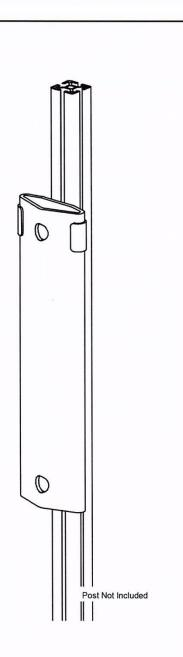
Post Mounting- Slide the T-nuts into the slots of the Gridiron post, tighten when in the desired location.
